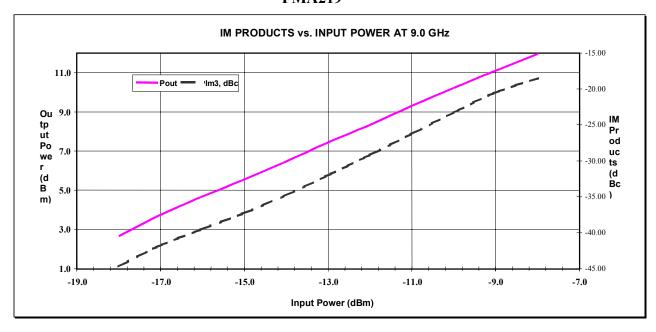
➤ Equivalent output IP3 performance exceeds 24 dBm, input IP3 is typically ≥ +2 dBm.
