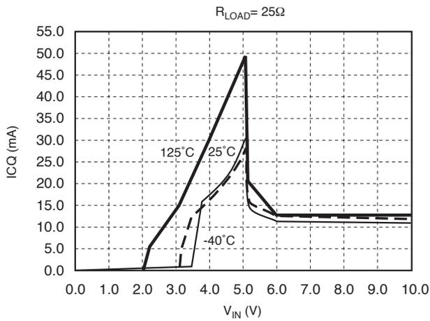
I<sub>CQ</sub> vs. V<sub>IN</sub> over R<sub>LOAD</sub>
