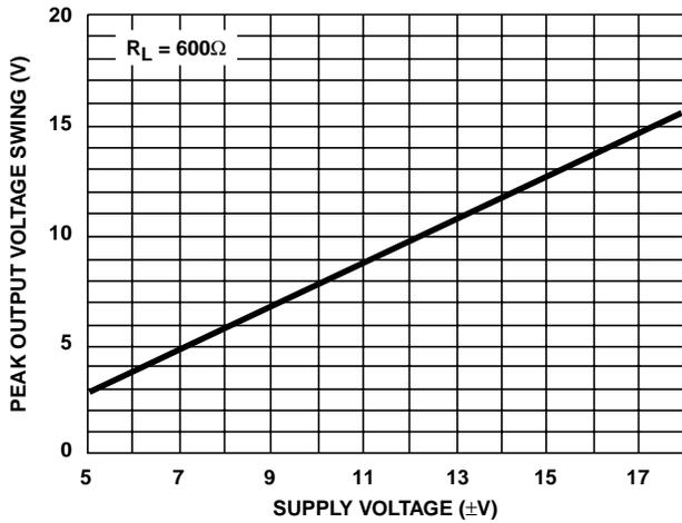
FIGURE 19. OUTPUT VOLTAGE SWING vs SUPPLY VOLTAGE
