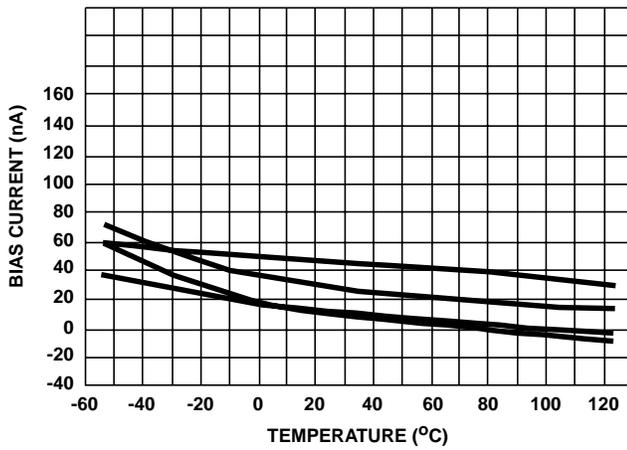
FIGURE 13. BIAS CURRENT vs TEMPERATURE (4 REPRESENTATIVE UNITS)
