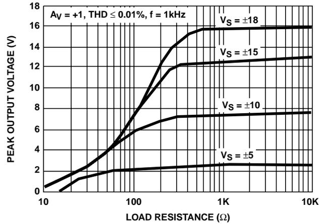
FIGURE 28. OUTPUT VOLTAGE SWING vs LOAD RESISTANCE
