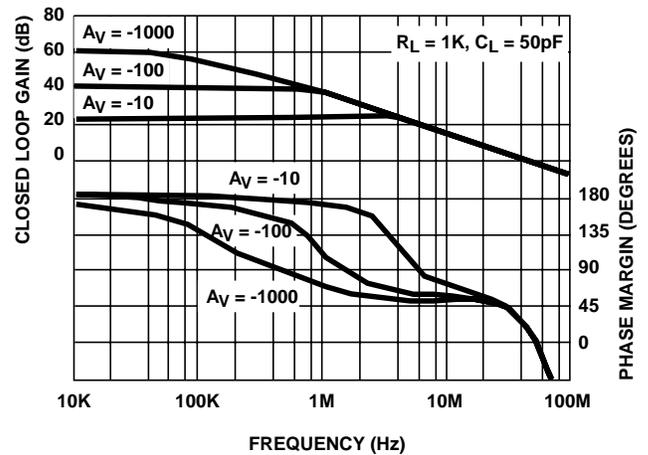
FIGURE 8. VARIOUS CLOSED LOOP GAINS vs FREQUENCY
