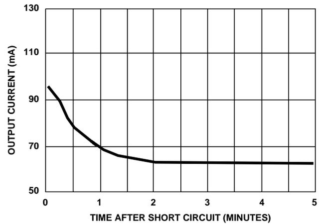
FIGURE 24. SHORT CIRCUIT OUTPUT CURRENT vs TIME
