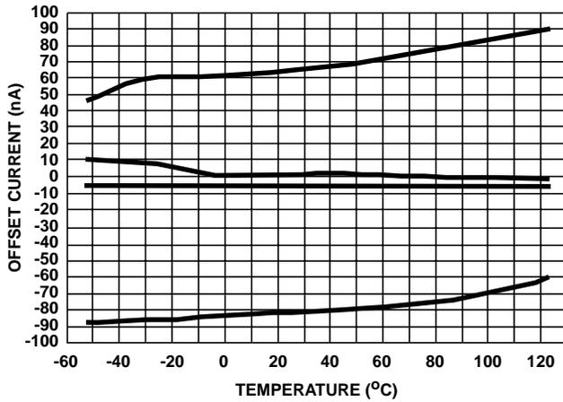
FIGURE 21. OFFSET CURRENT vs TEMPERATURE (4 REPRESENTATIVE UNITS)
