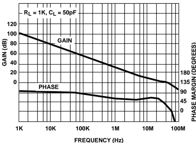
FIGURE 5. OPEN LOOP GAIN AND PHASE vs FREQUENCY
