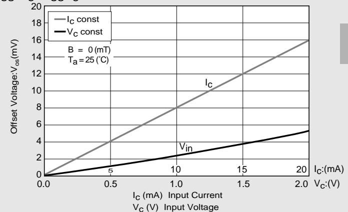
In This Example :  $R_{in}=340(\Omega)$ ,  $V_{os}=2.4\text{mV}$ ,  $V_C=1\text{V}$
