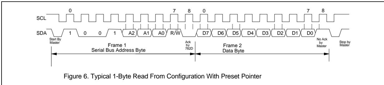
Figure 6. Typical 1-Byte Read From Configuration With Preset Pointer
