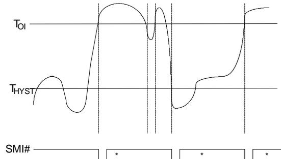
Figure 15-2. Two-Times Interrupt Mode
