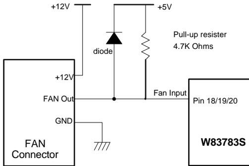
Figure 13-1. Fan with Tach Pull-Up to +5V
