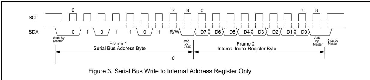
**6.2.2 The serial bus timing of the temperature 2 and 3 is shown as follow:**
