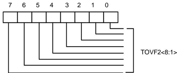
Bit 7-0: Over-temperature bit 8-1, which is High Byte. The temperature default 80 degree C.
