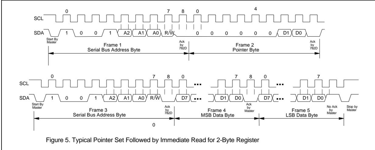
Figure 5. Typical Pointer Set Followed by Immediate Read for 2-Byte Register
