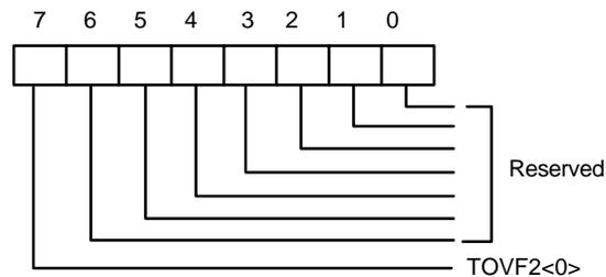
Bit 7: Read/Write - Over-temperature bit 0, which is low Byte.
