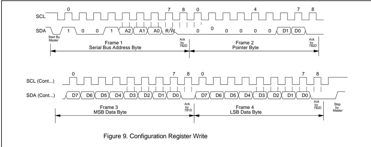
Figure 9. Configuration Register Write
