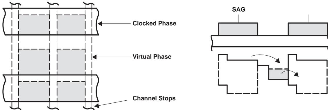
Figure 2. Charge-Transfer Process
