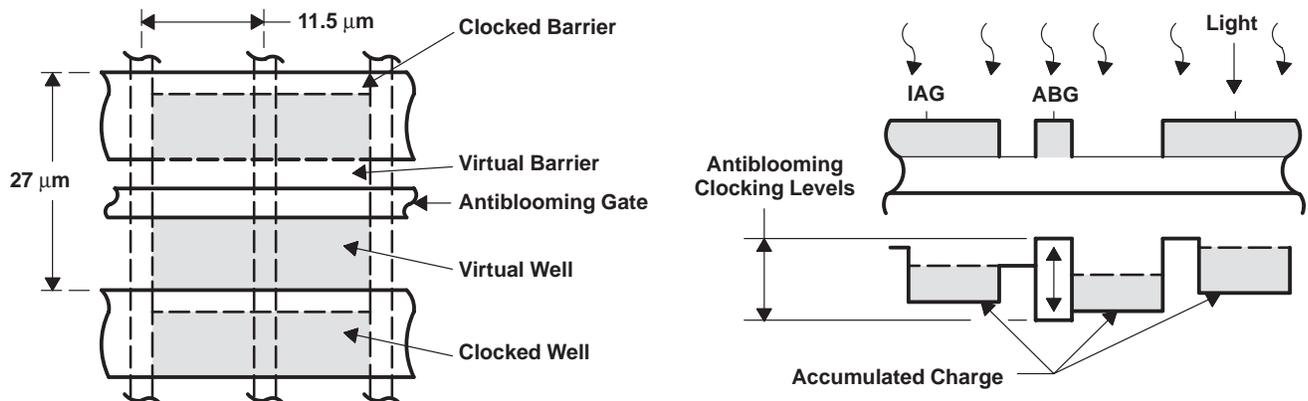
Figure 1. Charge-Accumulation Process
