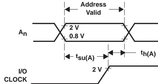
Figure 3. Address Timing
