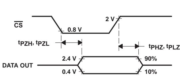
Figure 2.  $\overline{\text{CS}}$  to Data Output Timing
