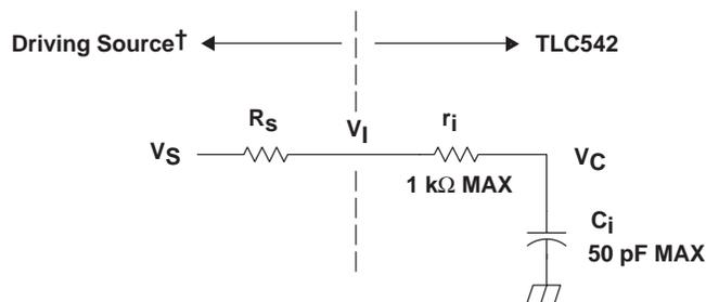
$V_I$  = Input Voltage at INPUT A0–A10
