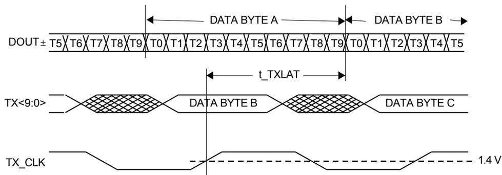
**Figure 4. Transmitter Latency**
