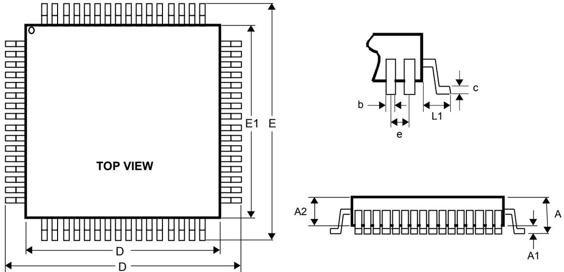
Figure 7. Mechanical Dimensions
