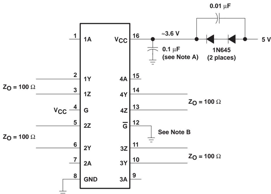
NOTE A: Place a 0.1 μF Z5U ceramic, mica or polystyrene dielectric, 0805 size, chip capacitor between V<sub>CC</sub> and the ground plane. The capacitor should be located as close as possible to the device terminals.
