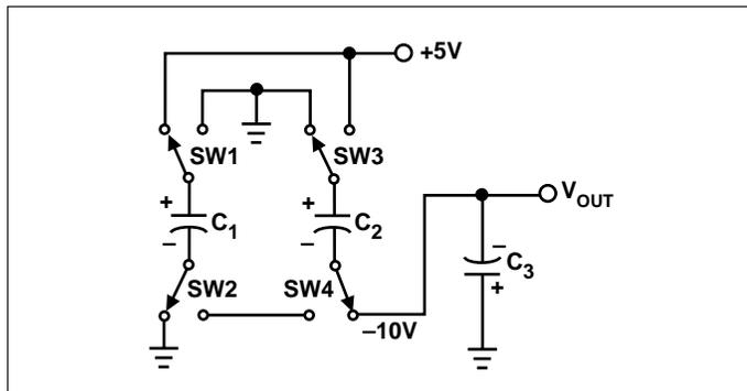
Figure 3. Charge Pump – Phase 2
