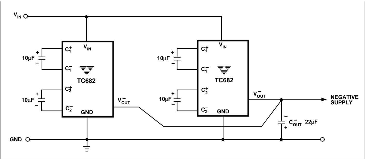
Figure 5. Paralleling TC682 for Lower Output Source Resistance
