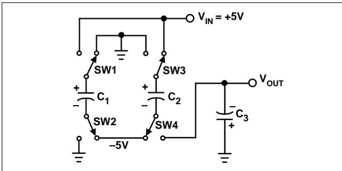
Figure 2. Charge Pump – Phase 1
