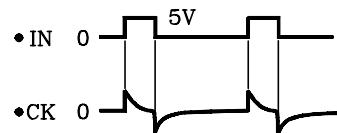
The capacitor coupling allows reset pulses to be supplied intermittently from the  $\overline{\text{RESET}}$  pin whether the input level (IN) is high or low.
