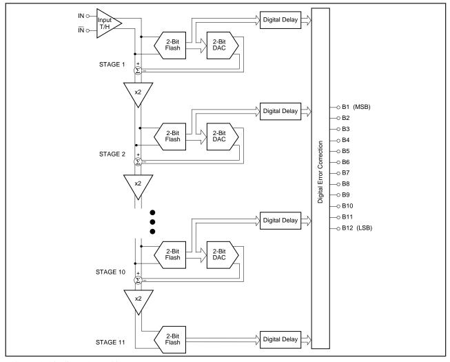
FIGURE 2. Pipeline A/D Architecture.
