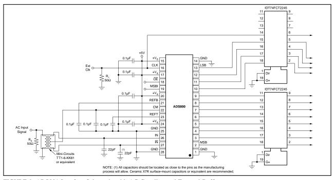
FIGURE 9. ADS801 Interface Schematic with AC-Coupling and External Buffers.
