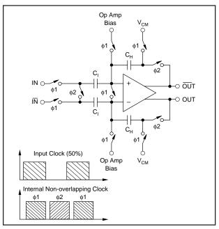
FIGURE 1. Input Track/Hold Configuration with Timing Signals.
