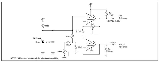
FIGURE 8. Optional External Reference to Set the Full-Scale Range Utilizing a Dual, Single-Supply Op Amp.
