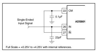
FIGURE 7. Single-Ended Input Connection.
