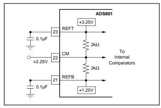
FIGURE 3. Internal Reference Structure.
