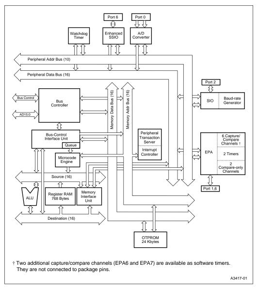
Figure 1. 87C196LA Block Diagram
