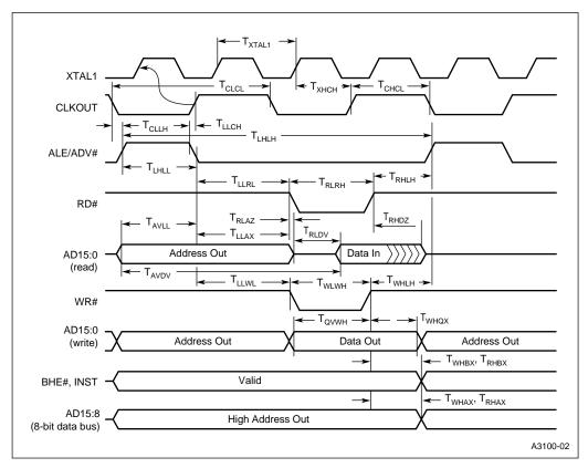
Figure 4. System Bus Timing
