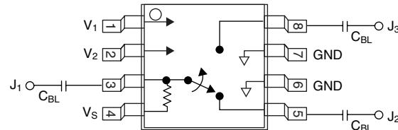
DC blocking capacitors (C<sub>BL</sub>) must be supplied externally.
