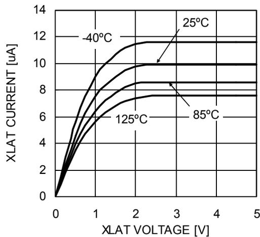
**BLANK pull-up Current vs. Input Voltage**
