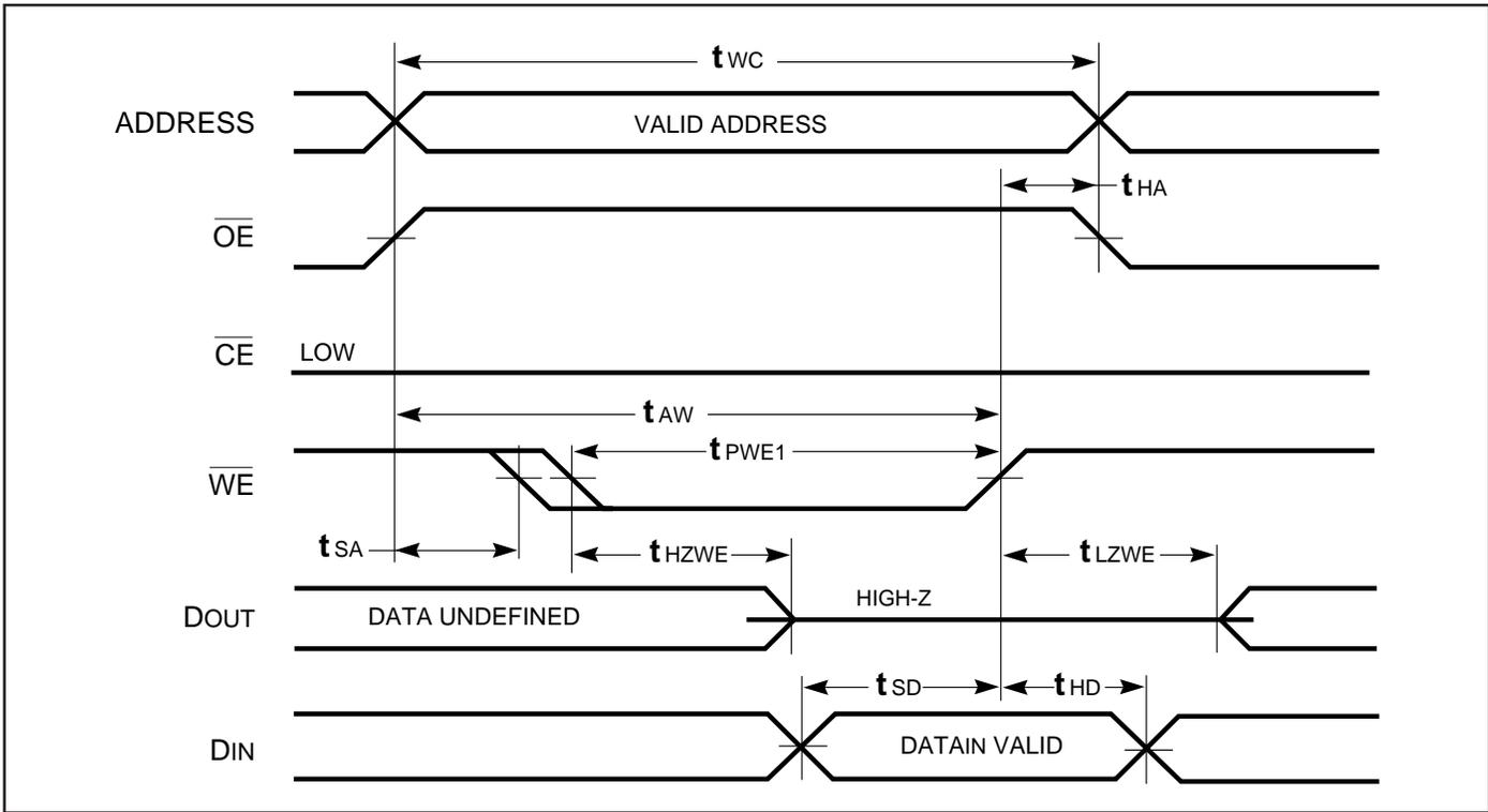
**WRITE CYCLE NO. 3** ( $\overline{WE}$  Controlled,  $\overline{OE}$  is LOW During Write Cycle) <sup>(1)</sup>
