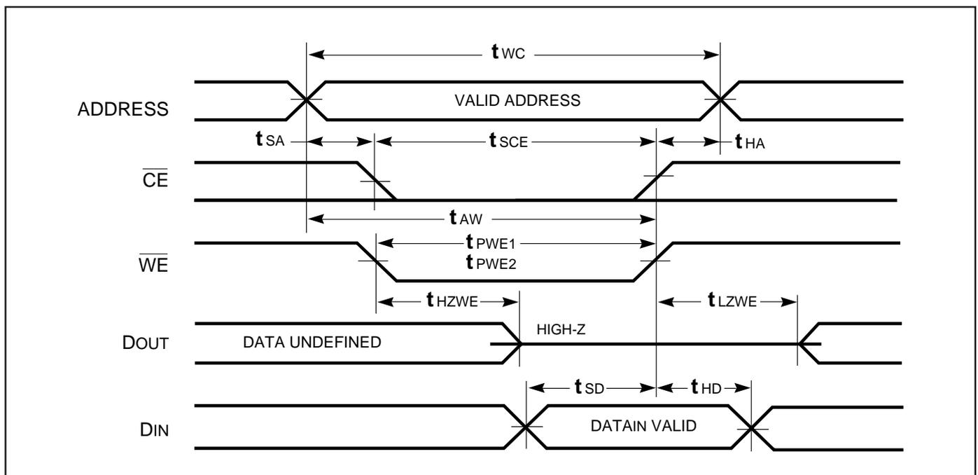
**WRITE CYCLE NO. 2** ( $\overline{WE}$  Controlled,  $\overline{OE}$  is HIGH During Write Cycle) <sup>(1,2)</sup>
