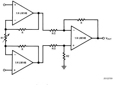
$$V_{OUT}=2{\left(\frac{2R}{R1}+1\right)}, V_{\overline{S}}-3V\leq V_{IN\,CM}\leq {V_S}^+-3V,$$
