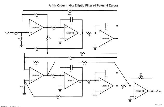
$$\label{eq:rescaled} \begin{split} R1C1 &= R2C2 = t \\ R'1C'1 &= R'2C'2 = t' \\ f_C &= 1 \ \text{kHz}, \ f_S &= 2 \ \text{kHz}, \ f_p = 0.543, \ f_Z &= 2.14, \ Q &= 0.841, \ f'_P &= 0.987, \ f'_Z &= 4.92, \ Q' &= 4.403, \ \text{normalized to ripple BW} \end{split}$$
