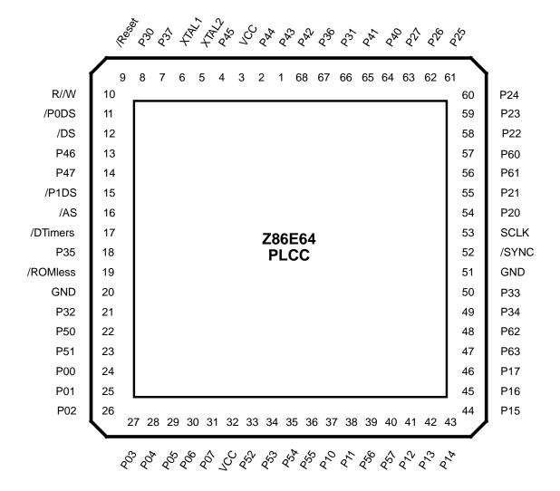
Figure 2. Z86E64 68-Pin PLCC Pin Assignments
