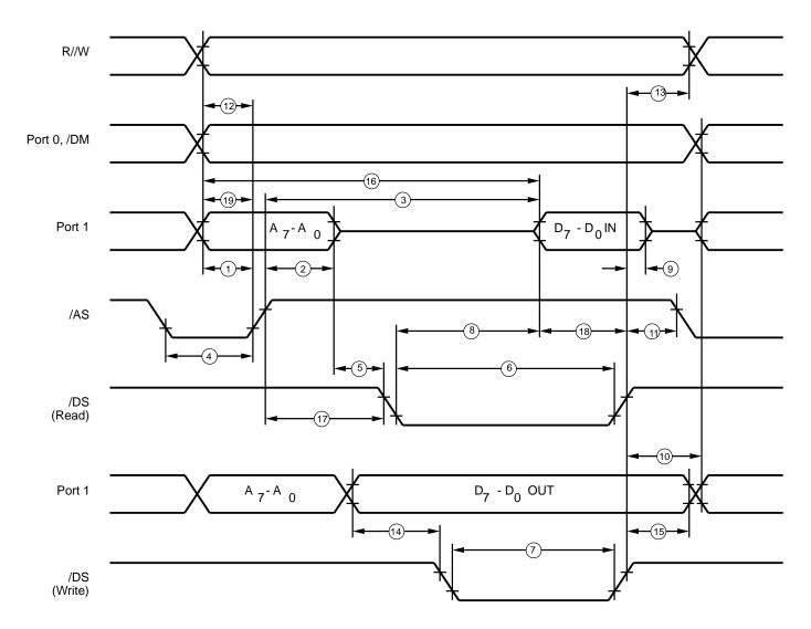
Figure 3. External I/O or Memory Read/Write Timing
