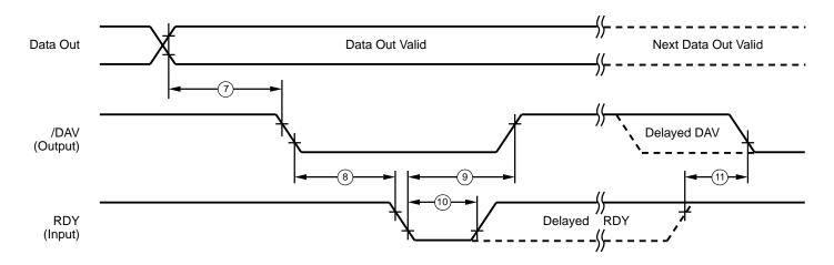
Figure 6. Output Handshake Timing
