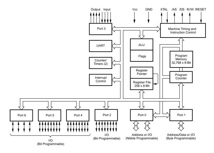
Figure 1. Z86E64 Functional Block Diagram
