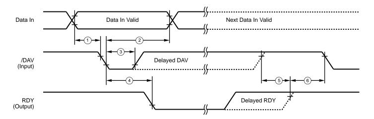
Figure 5. Input Handshake Timing
