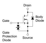
Remark The diode connected between the gate and source of the transistor serves as a protector against ESD.
