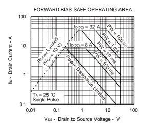
**Remark** Mounted on ceramic substrate of  $1200 \text{ mm}^2 \times 2.2 \text{ mm}$
