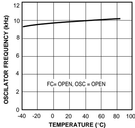
12) Oscillator Frequency vs. Temperature
