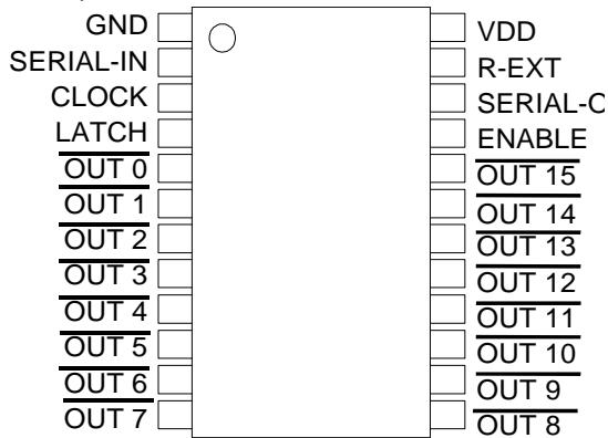
Warnings : Short-circuiting an output terminal to GND or to the power supply terminal may broken the device.
