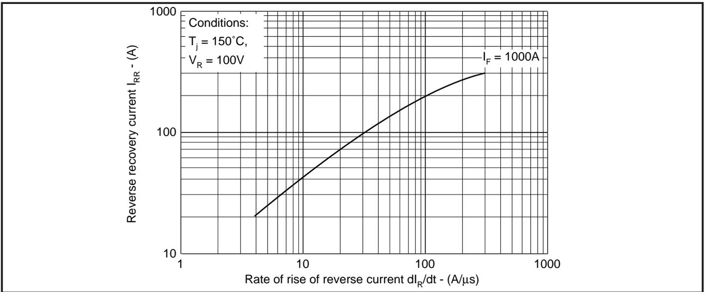
Fig.4 Typical reverse recovery current vs rate of rise of reverse current
