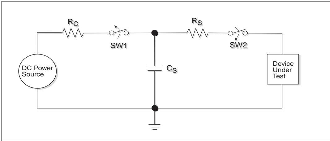
Figure 5. ESD Test Circuit for Human Body Model
