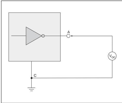
**Figure 12. V.28 Driver Output Open Circuit Voltage**
