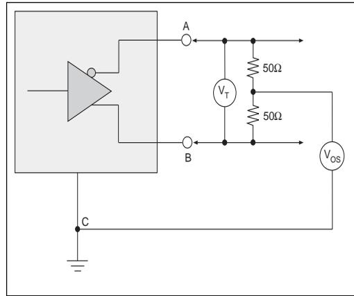
**Figure 2. V.35 Driver Output Test Terminated Voltage**
