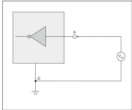
**Figure 19. V.28 Receiver Input Open Circuit Bias**
