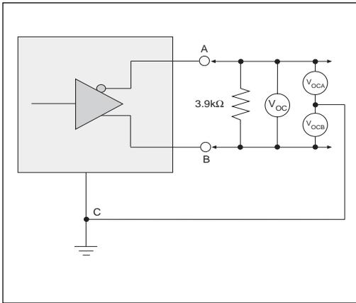
**Figure 1. V.11 and V.35 Driver Output Open-Circuit Voltage**
