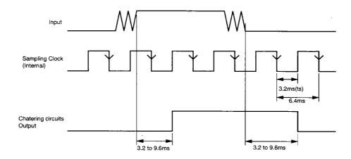
Note that the input is recognized during the LOW-level pulse interval,  $t_S$  (32 ms), of the sampling clock.
