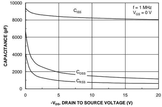
Figure 8. Capacitance Characteristics.
