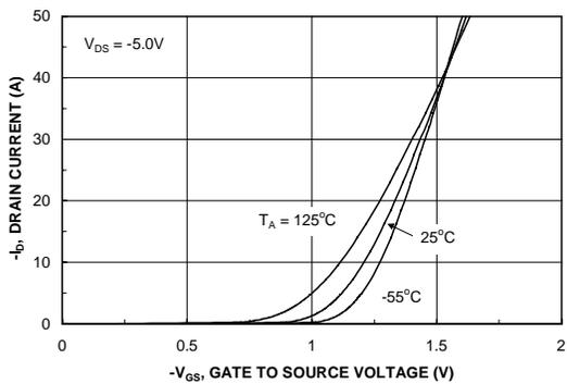
Figure 5. Transfer Characteristics.
