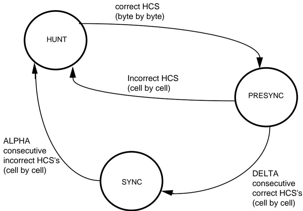
The values of ALPHA and DELTA determine the robustness of the delineation process. ALPHA determines the robustness against false misalignments due to bit errors. DELTA determines the robustness against false delineation in the synchronization process. ALPHA is chosen to be 7 and DELTA is chosen to be 6. These values result in an average time to delineation of 8  $\mu$ s for the STS-12c/STM-4-4c rate.
