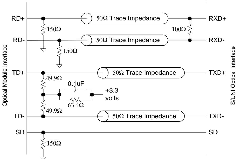
**Figure 27: Interfacing S/UNI-622-MAX PECL Pins to 5.0V Devices**
