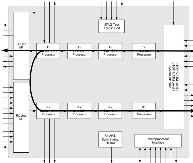
**Figure 19: Path Diagnostic Loopback Mode**
