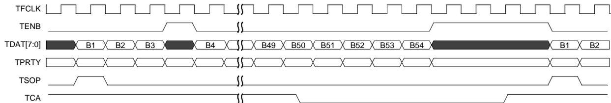
The Receive UTOPIA Level 3 System Interface Timing diagram (Figure 34) illustrates the operation of the system side receive interface. Unlike traditional UTOPIA interfaces, the SUNI-622-MAX controls the bus. Because the bus is point to point, the SUNI-622-MAX pushes received data to the downstream reader. As well, the control of RENB is pipelined to improve the speed of the interface.
