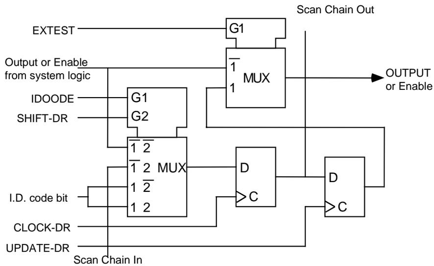
**Figure 9: Bidirectional Cell (IO\_CELL)**
