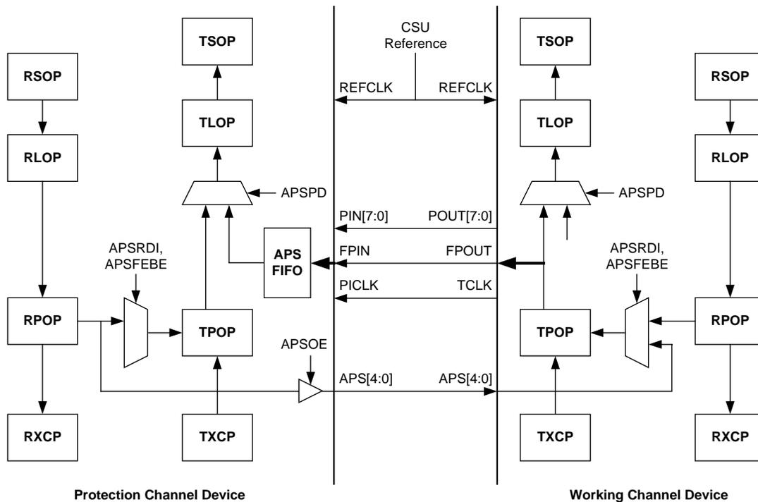
A 4-byte FIFO is used to handle wander between the TCLK of the working device and the TCLK of the protection device. Both transmit clocks TCLK must be the same frequency in order for this FIFO to operate normally. Therefore, the clock synthesis units (CSU) of both device must have the same reference clock input
