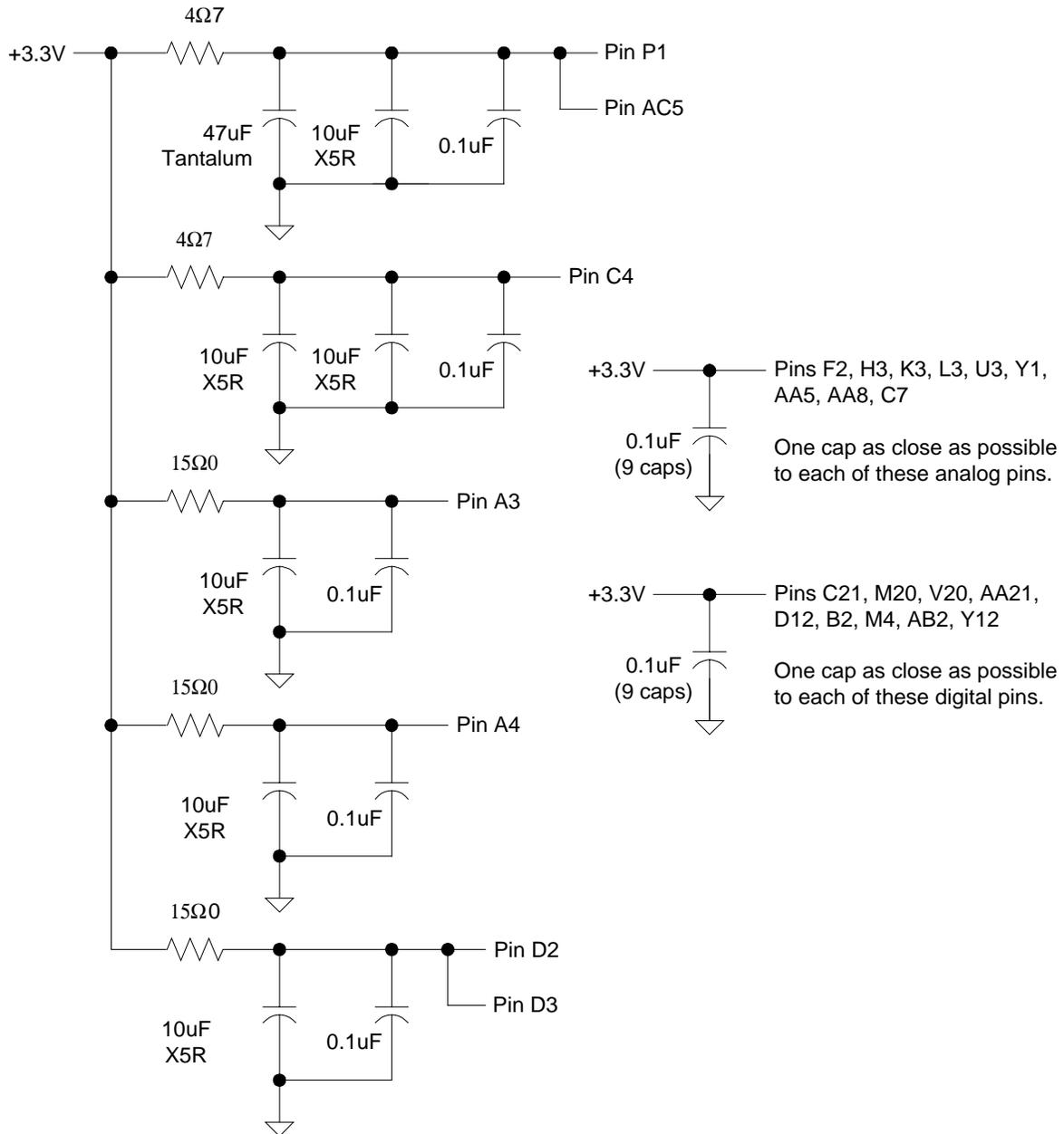
**Figure 25: Power Supply Component Layout**
