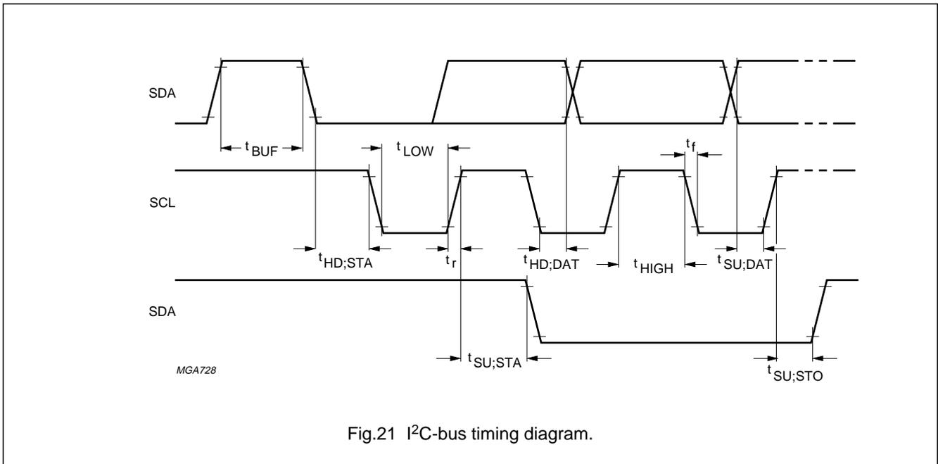
Fig.21 I<sup>2</sup>C-bus timing diagram.
