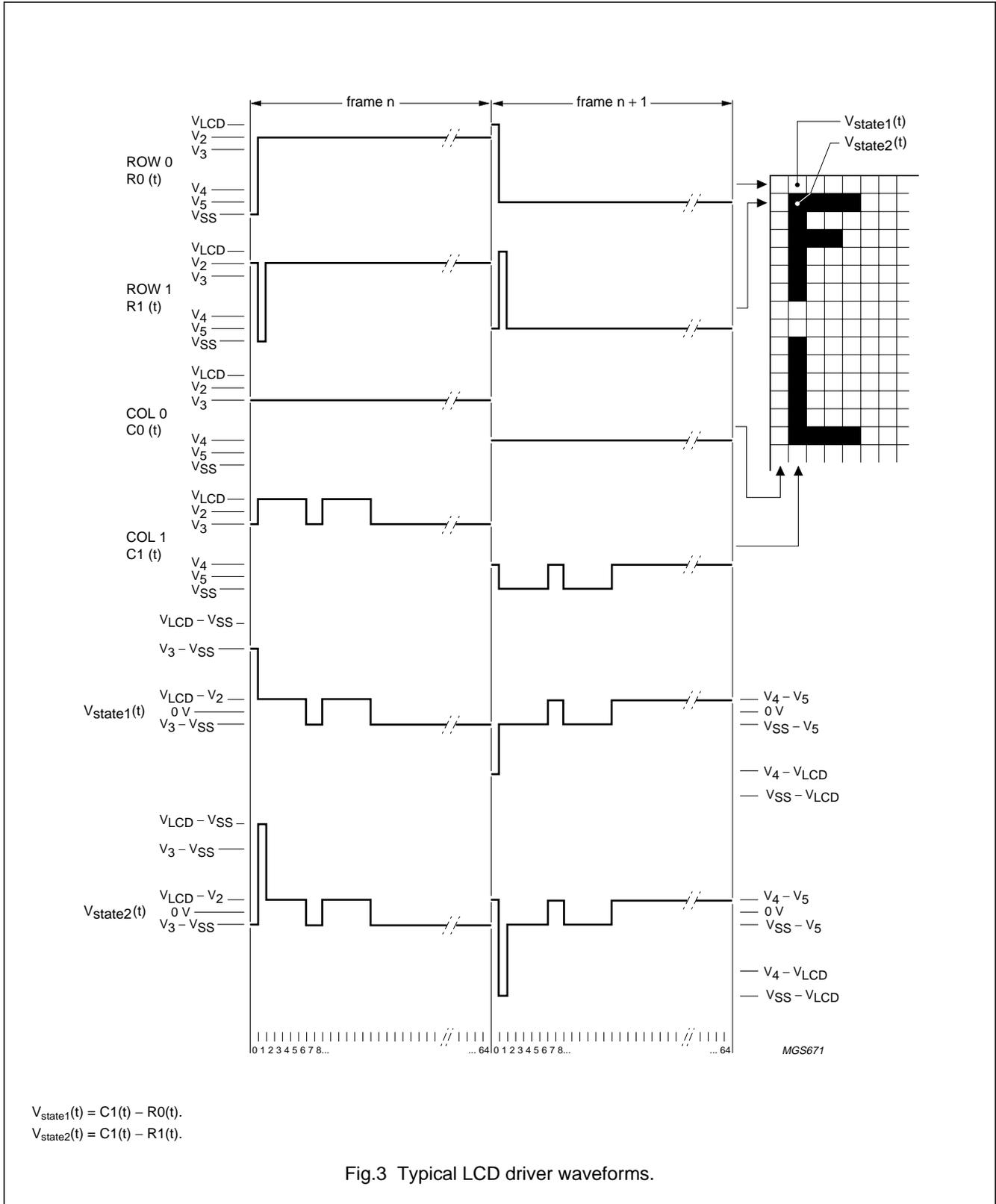
Fig.3 Typical LCD driver waveforms.
