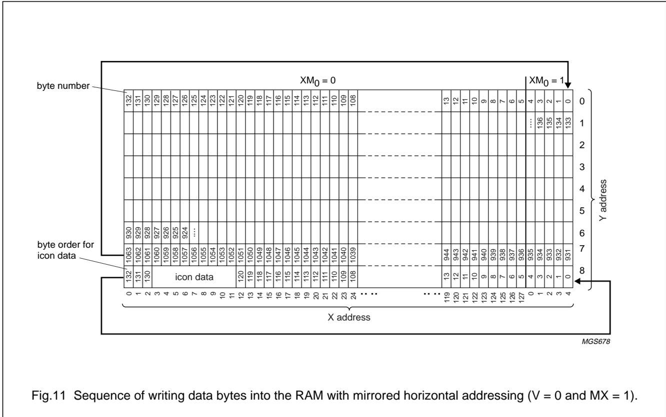
Fig.11 Sequence of writing data bytes into the RAM with mirrored horizontal addressing (V = 0 and MX = 1).
