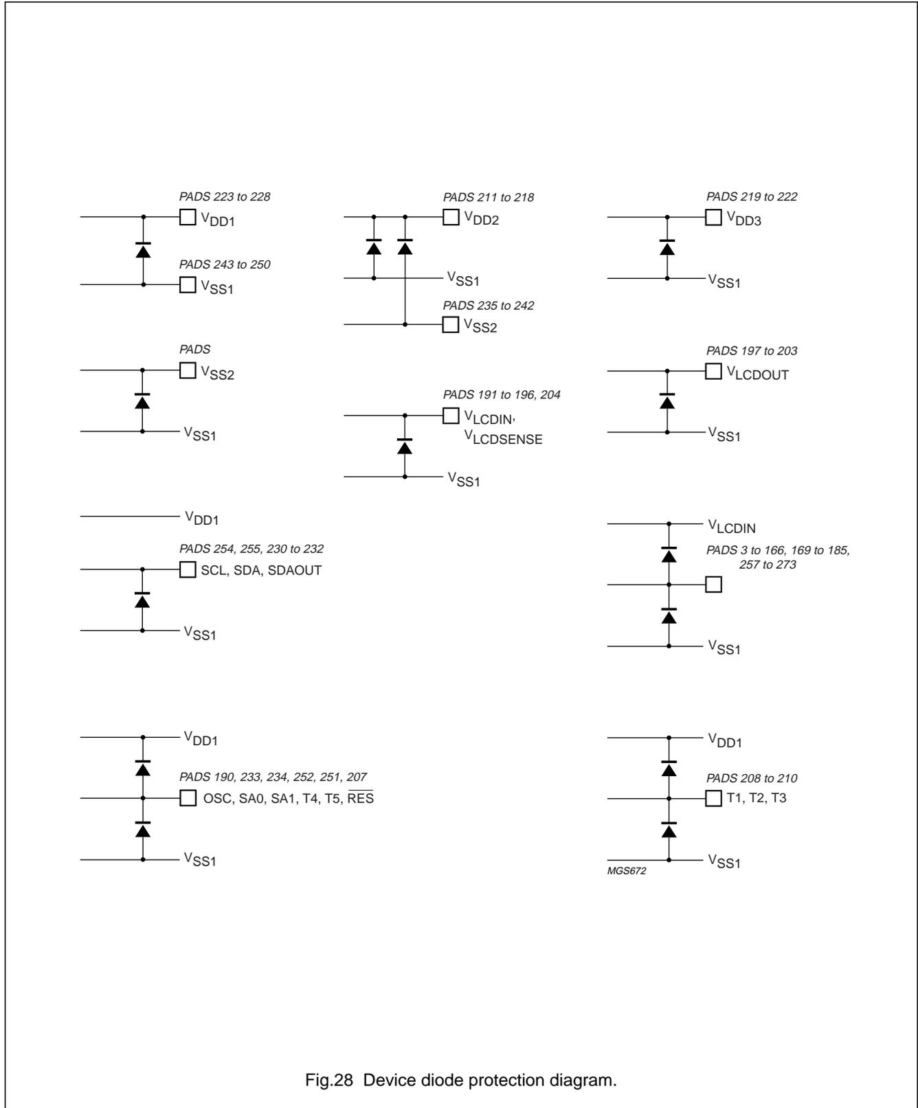
Fig.28 Device diode protection diagram.
