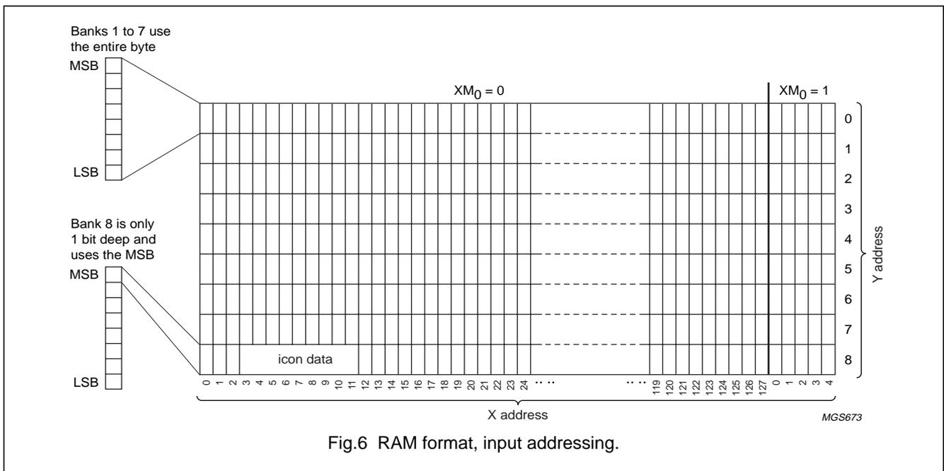
Fig.6 RAM format, input addressing.
