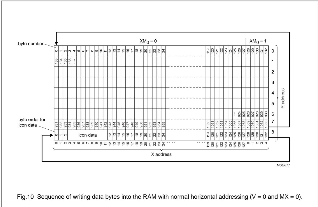
Fig.10 Sequence of writing data bytes into the RAM with normal horizontal addressing (V = 0 and MX = 0).
