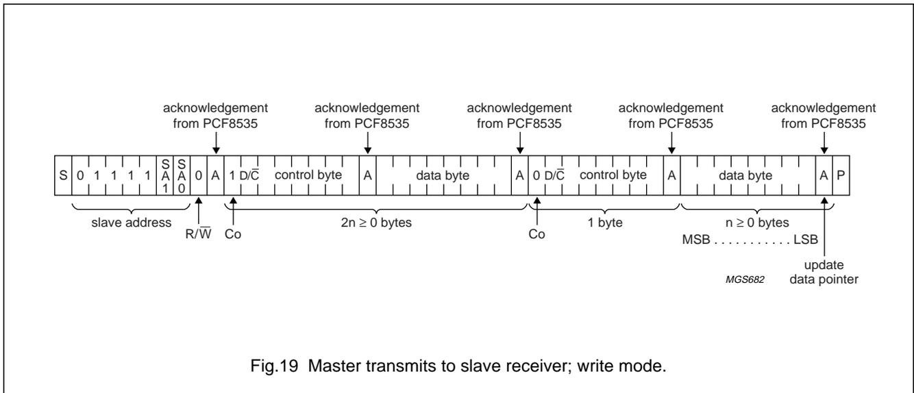
Fig.19 Master transmits to slave receiver; write mode.
