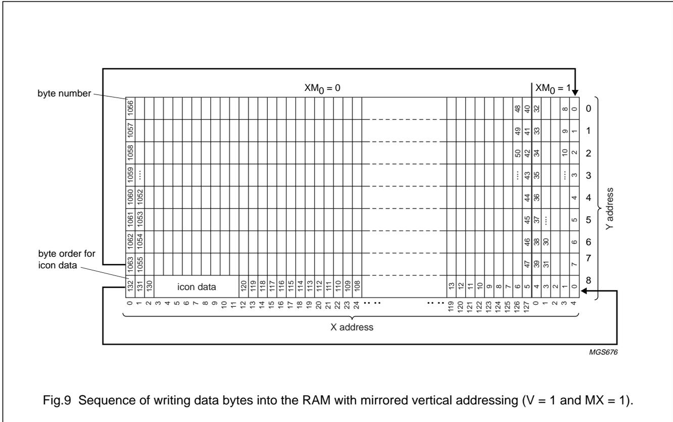
Fig.9 Sequence of writing data bytes into the RAM with mirrored vertical addressing (V = 1 and MX = 1).
