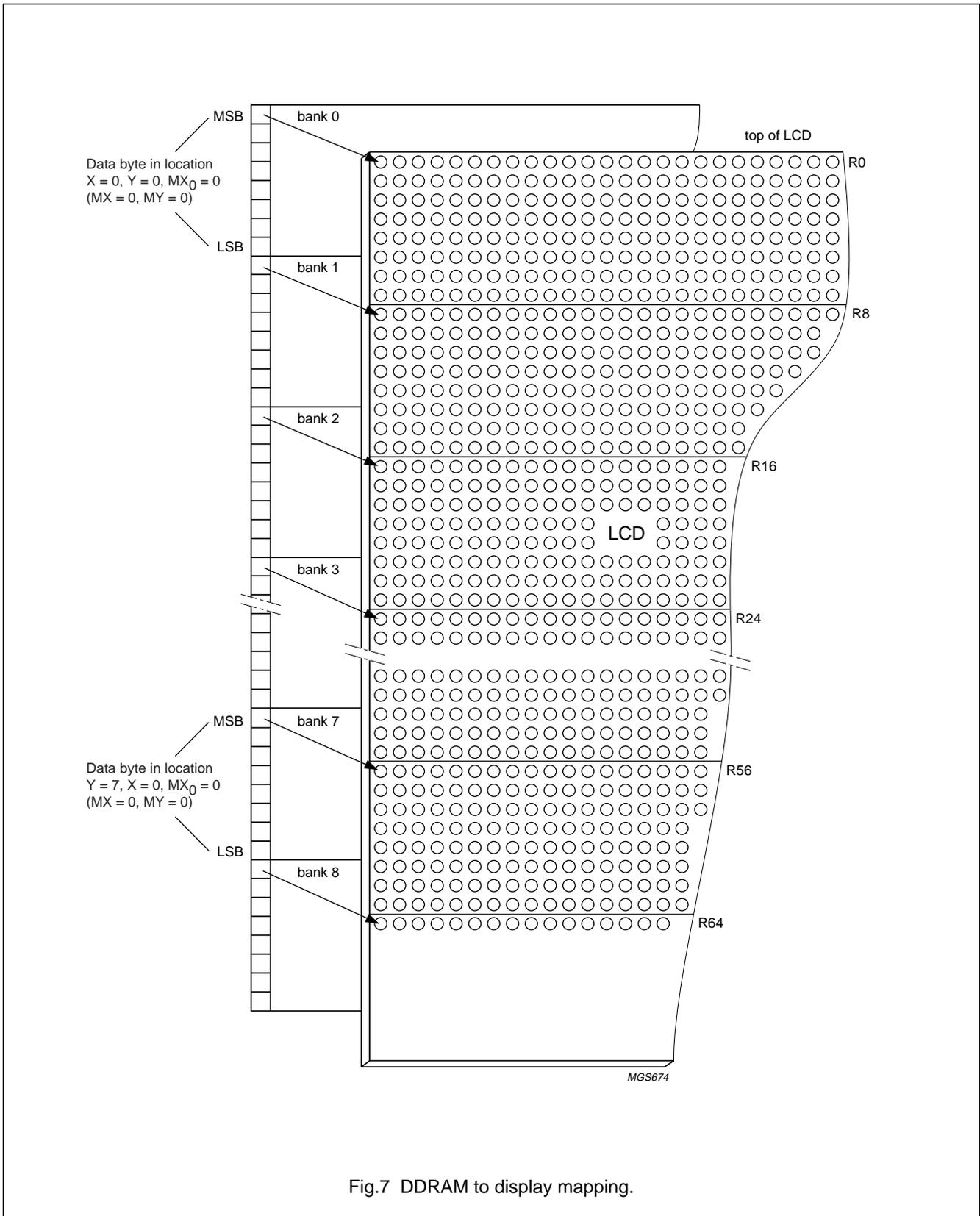
Fig.7 DDRAM to display mapping.
