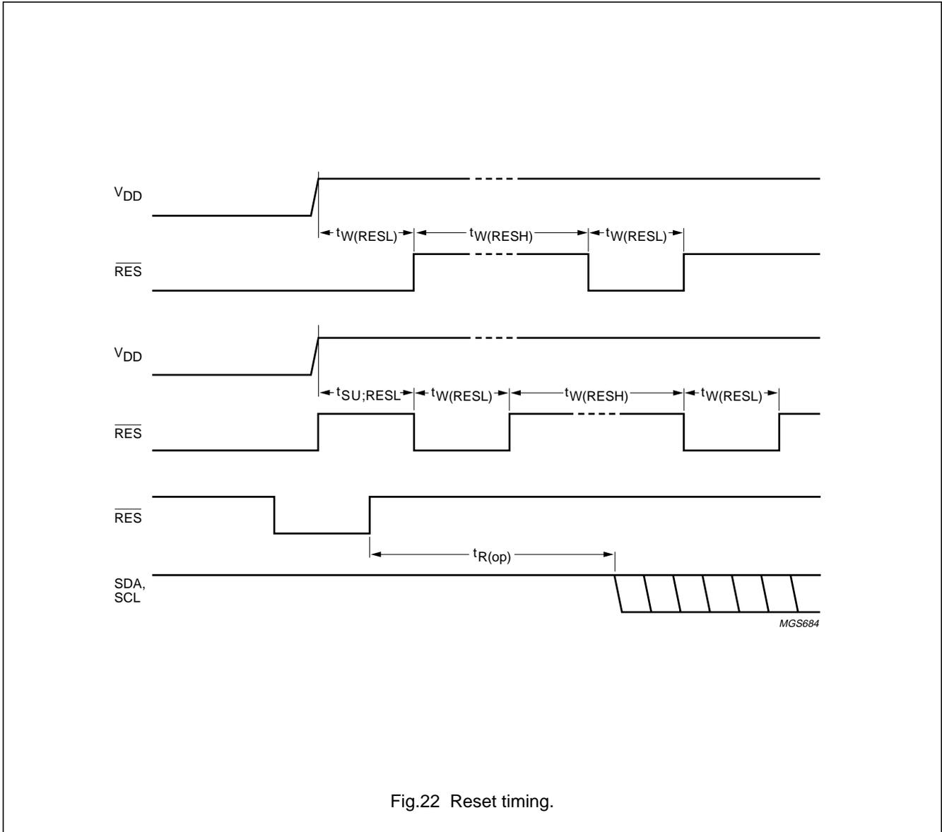
Fig.22 Reset timing.
