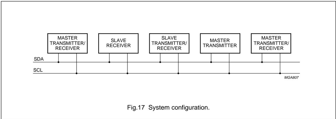
Fig.17 System configuration.
