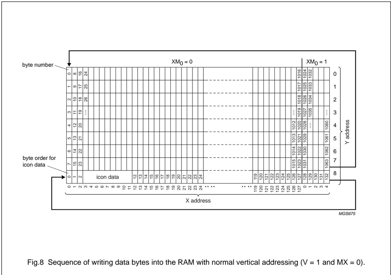
Fig.8 Sequence of writing data bytes into the RAM with normal vertical addressing ( $V = 1$  and  $MX = 0$ ).
