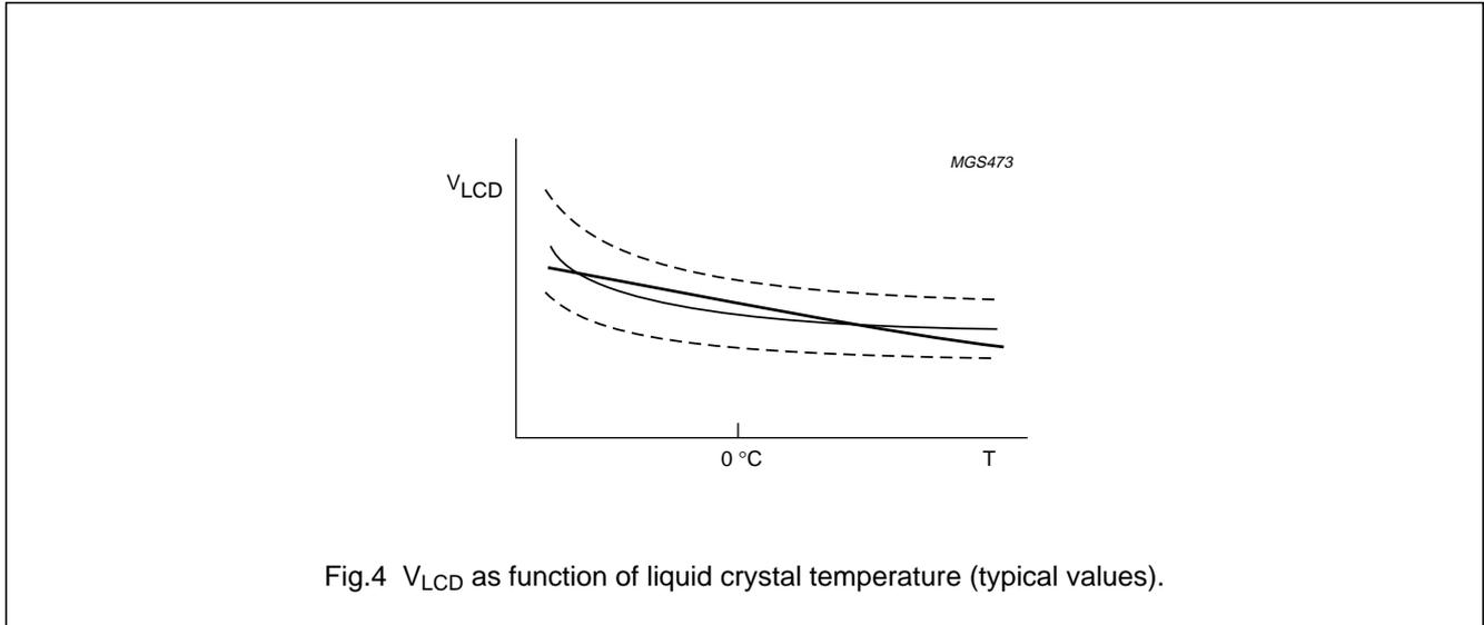
Fig.4 V<sub>LCD</sub> as function of liquid crystal temperature (typical values).
