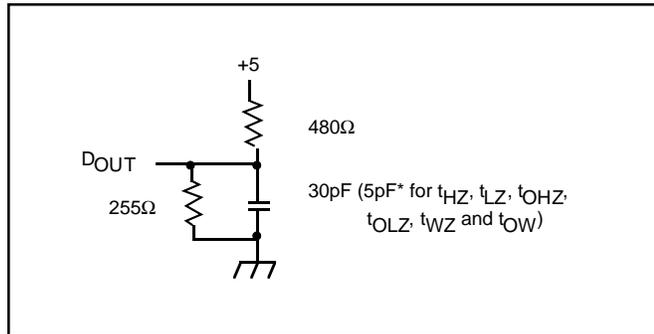
Figure 1. Output Load
