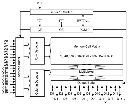
In 8-bit output mode, these pins are three-stated and pin D15 functions as the A-1 address pin.
