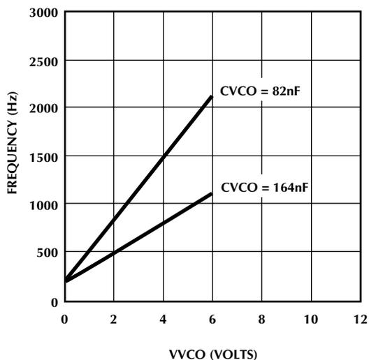
Figure 3. VCO Output Frequency vs.  $V_{VCO}$  (Pin 20)
