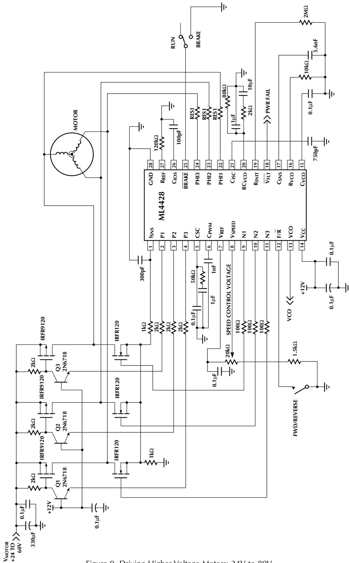
Figure 9. Driving Higher Voltage Motors: 24V to 80V.
