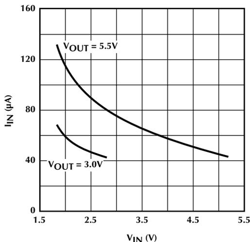
Figure 6. No Load Input Current vs.  $V_{IN}$
