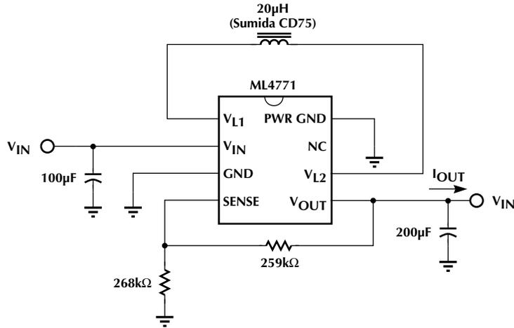
Figure 1. Application Test Circuit.
