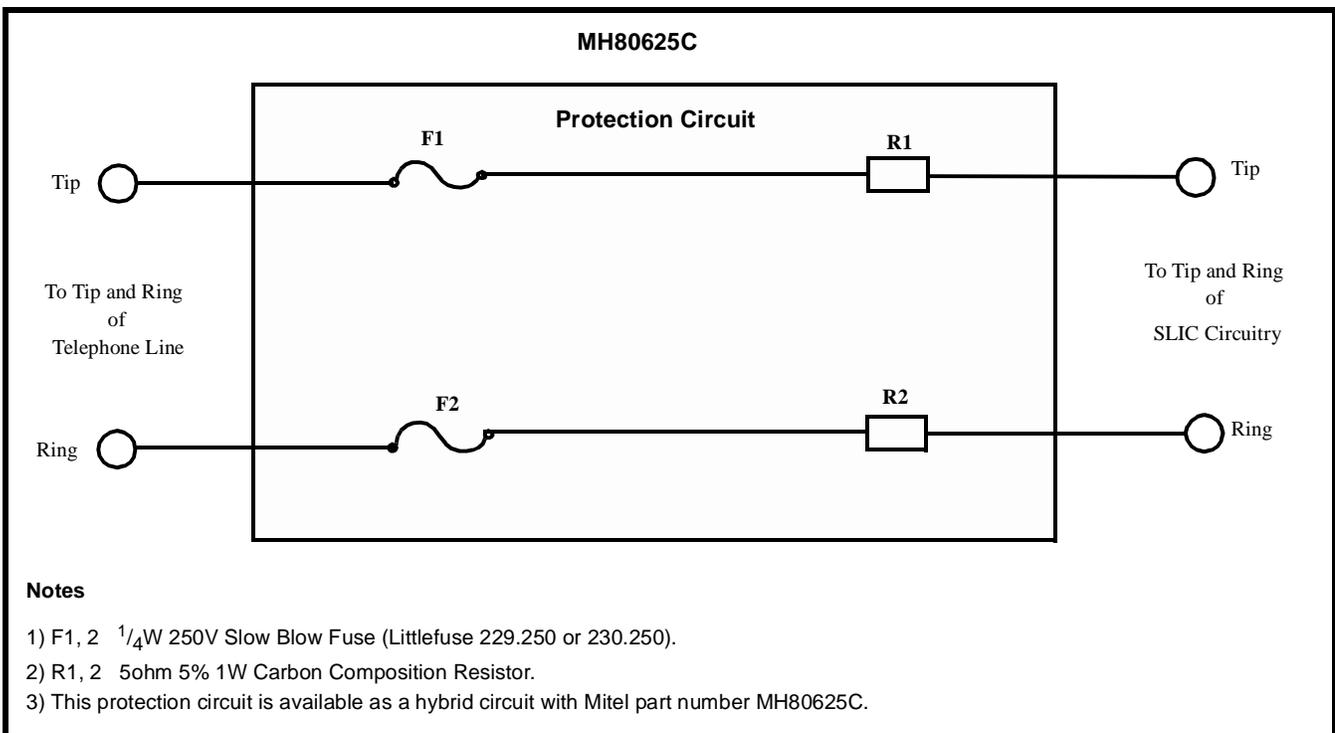
Figure 5 - Solid State External Protection Application Circuit
