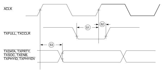
Figure 19. Transmit PHY Interface Timing
