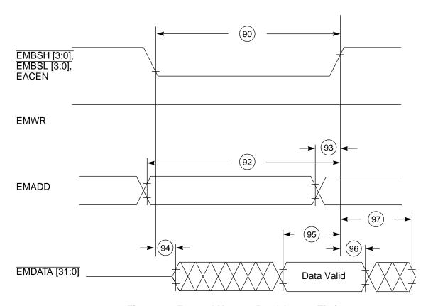
Figure 23. External Memory Read Access Timing
