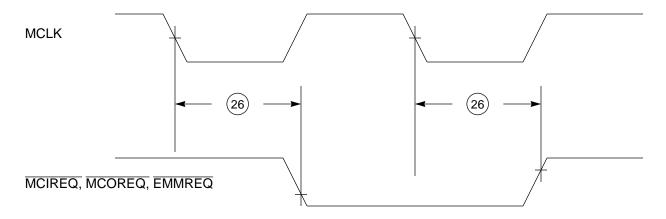
Figure 17. DMA Request Signals Timing
