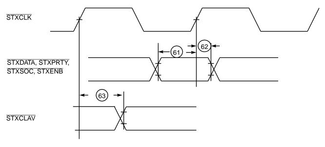
Figure 21. Egress Switch Interface Timing
