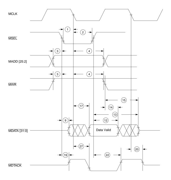
Figure 14. General Register Read Access Timing
