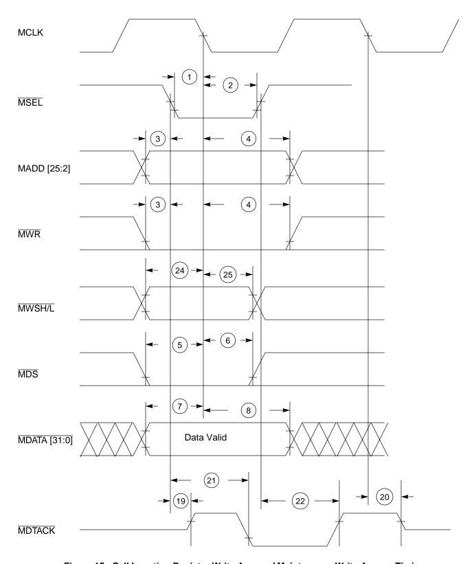
Figure 15. Cell Insertion Register Write Access / Maintenance Write Access Timing
