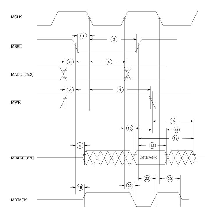
Figure 13. Maintenance Read Access Timing
