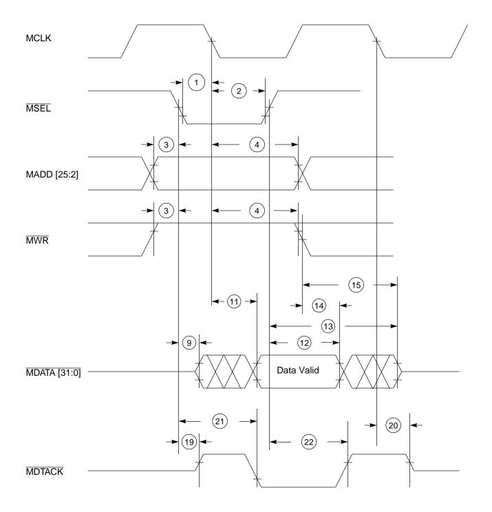
Figure 12. Cell Extraction Register Read Access Timing
