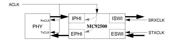
Figure 10. MC92500 Clock Configuration
