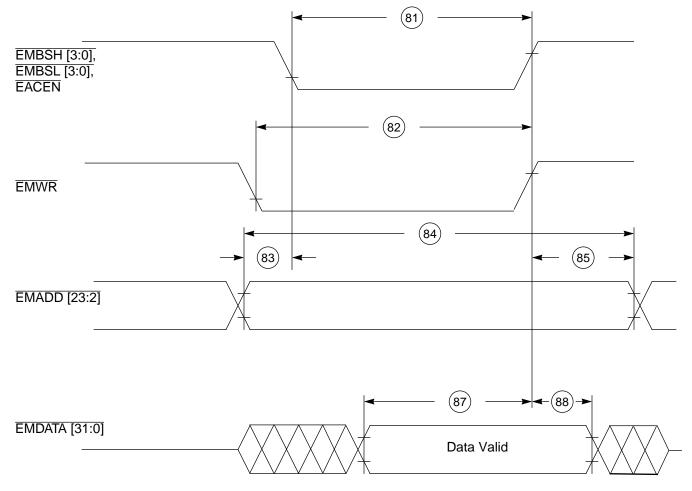
Figure 22. External Memory Write Access Timing
