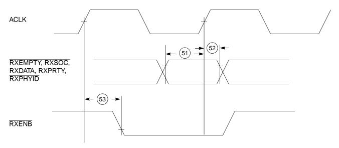
Figure 18. Receive PHY Interface Timing
