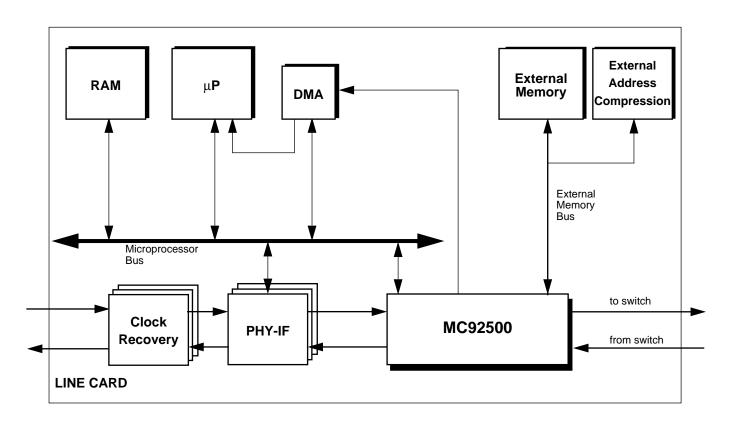
Figure 3. Typical MC92500 Line Card Application
