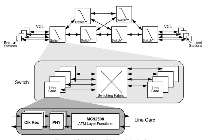
Figure 2. MC92500 in an ATM Network Application
