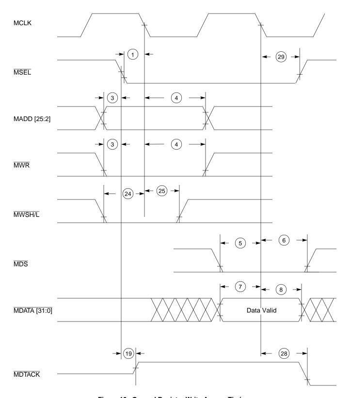
Figure 16. General Register Write Access Timing
