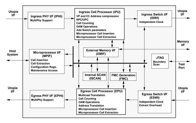
Figure 4. MC92500 Block Diagram
