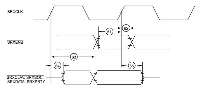
Figure 20. Ingress Switch Interface Timing
