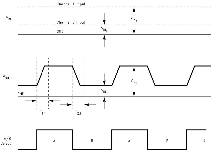
**FIGURE 1. Rise and Fall Times at Outputs**
