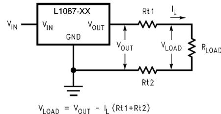
FIGURE 2. Typical Application using Fixed Output Regulator
