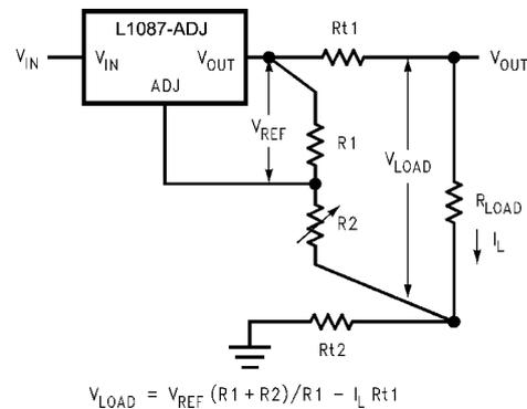
FIGURE 3. Best Load Regulation using Adjustable Output Regulator
