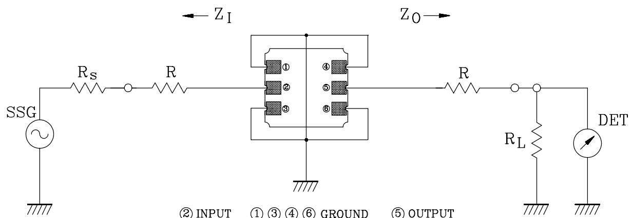
$R_S, R_L : 50\Omega$  (Internal Impedance of Source and Load)
