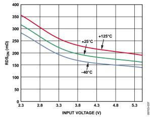
Figure 32. NMOS RDS<sub>ON</sub> vs. Input Voltage Across Temperature
