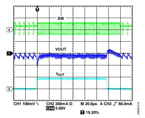
Figure 28. BUCK2 Response to Load Transient,  $I_{OUT2}$  = 20 mA to 180 mA,  $V_{OUT2}$  = 1.8 V, Auto Mode
