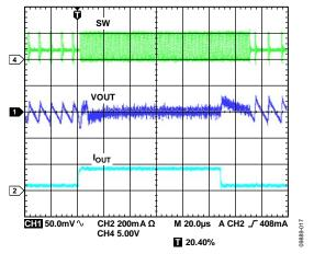
Figure 27. BUCK1 Response to Load Transient,  $I_{OUT1} = 20$  mA to 180 mA,  $V_{OUT1} = 3.3$  V, Auto Mode
