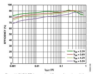
Figure 11. BUCK2 Efficiency vs. Load Current, Across Input Voltage,  $V_{\text{OUT2}}$  = 1.8 V, Auto Mode
