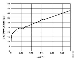
Figure 36. LDO Ground Current vs. Output Load,  $V_{IN3} = 3.3 \text{ V}$ ,  $V_{OUT3} = 2.8 \text{ V}$
