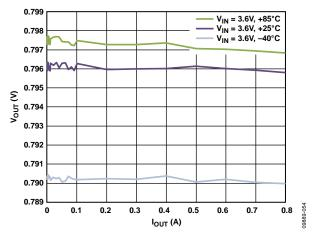
Figure 8. BUCK1 Load Regulation Across Input Voltage,  $V_{OUT1} = 3.3 V$ , PWM Mode
