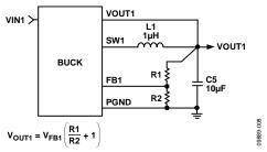
Figure 47. BUCK1 External Output Voltage Setting
