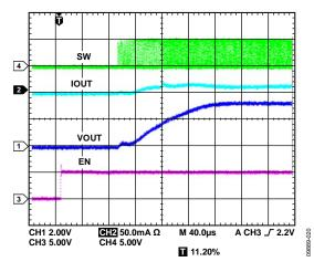
Figure 5. BUCK2 Startup,  $V_{\text{OUT2}} = 3.3 \text{ V}$ ,  $I_{\text{OUT2}} = 10 \text{ mA}$
