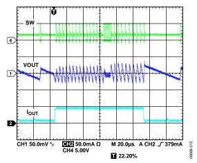
Figure 26. BUCK2 Response to Load Transient,  $I_{OUT2} = 1$  mA to 50 mA,  $V_{OUT2} = 1.8$  V, Auto Mode
