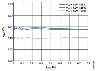
Figure 6. BUCK1 Load Regulation Across Temperature,  $V_{OUT1} = 3.3 V$ , Auto Mode
