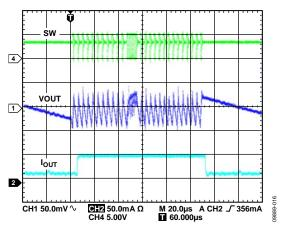
Figure 25. BUCK1 Response to Load Transient,  $I_{OUT1} = 1$  mA to 50 mA,  $V_{OUT1} = 3.3$  V, Auto Mode
