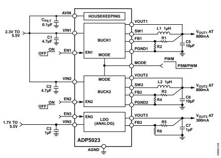
Figure 50. Processor System Power Management with PSM/PWM Control
