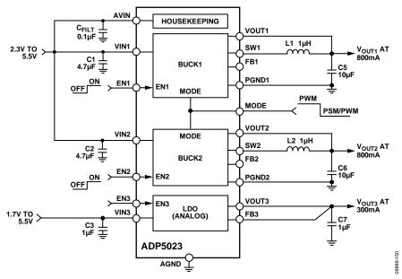
Figure 52. ADP5023 Fixed Output Voltages with Enable Pins
