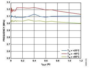
Figure 18. BUCK2 Switching Frequency vs. Output Current, Across Temperature,  $V_{\rm OUT2}$  = 1.8 V, PWM Mode
