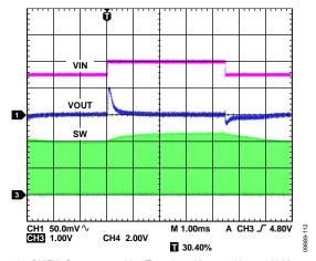
Figure 23. BUCK1 Response to Line Transient,  $V_{\rm IN}$  = 4.5 V to 5.0 V,  $V_{\rm OUT1}$  = 3.3 V, PWM Mode
