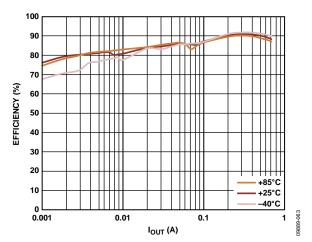
Figure 16. BUCK2 Efficiency vs. Load Current, Across Temperature,  $V_{\text{OUT2}} = 1.8 \text{ V}$ , Auto Mode
