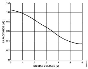
Figure 51. Capacitance vs. Voltage Characteristic
