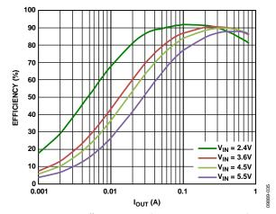
Figure 12. BUCK2 Efficiency vs. Load Current, Across Input Voltage,  $V_{OUZ} = 1.8 \text{ V}$ , PWM Mode
