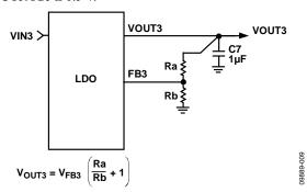
Figure 48. LDO External Output Voltage Setting
