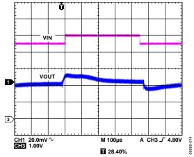
Figure 38. LDO Response to Line Transient,  $V_{IN} = 4.5 \text{ V}$  to 5.5 V,  $V_{OUT3} = 2.8 \text{ V}$
