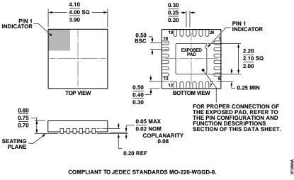
Figure 54. 24-Lead Lead Frame Chip Scale Package [LFCSP\_WQ] 4 mm × 4 mm Body, Very Very Thin Quad (CP-24-10) Dimensions shown in millimeters
