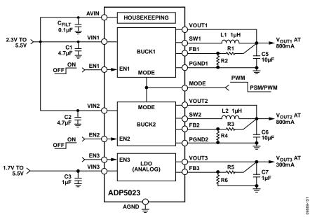
Figure 53. ADP5023 Adjustable Output Voltages with Enable Pins
