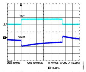
Figure 37. LDO Response to Load Transient,  $I_{OUT3} = 1$  mA to 80 mA,  $V_{OUT3} = 2.8$  V
