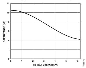
Figure 49. Capacitance vs. Voltage Characteristic
