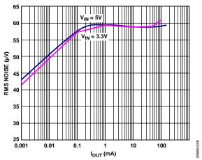
Figure 40. LDO Output Noise vs. Load Current, Across Input Voltage,  $V_{OU3} = 3.0 \text{ V}$
