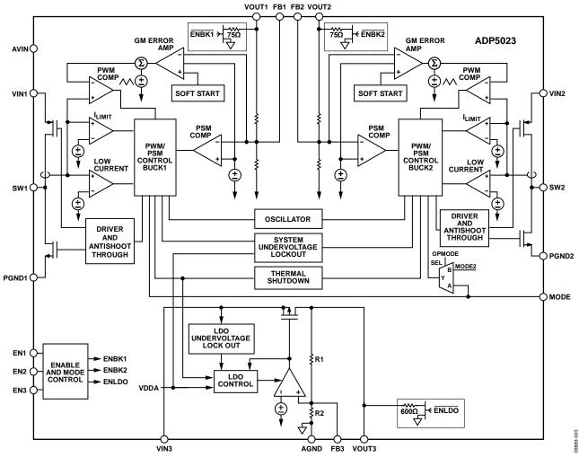
Figure 45. Functional Block Diagram
