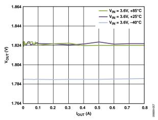
Figure 7. BUCK2 Load Regulation Across Temperature,  $V_{OUT2} = 1.8 V$ , Auto Mode
