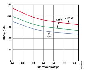
Figure 33. PMOS RDS<sub>ON</sub> vs. Input Voltage Across Temperature
