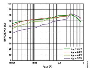
Figure 13. BUCK1 Efficiency vs. Load Current, Across Input Voltage, Vouti = 0.8 V, Auto Mode
