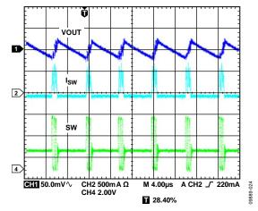
Figure 20. Typical Waveforms, V<sub>OUT2</sub> = 1.8 V, I<sub>OUT2</sub> = 30 mA, Auto Mode
