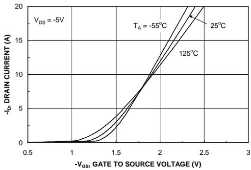
Figure 5. Transfer Characteristics.
