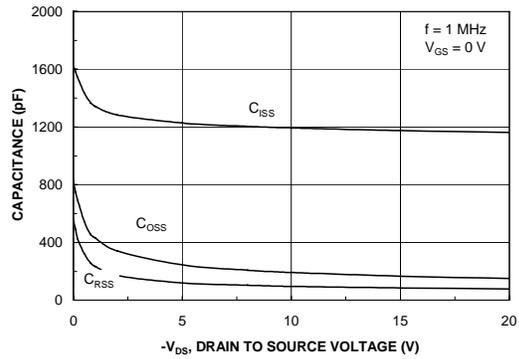
Figure 8. Capacitance Characteristics.
