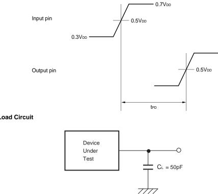
AC Testing Load Circuit
