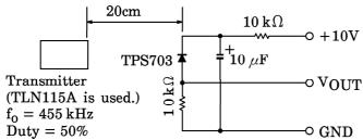
In the figure above, the transmitter output VOUT is 80 mVpp. The TPS703 in this application has a short-circuit current of  $I_{sc}=1.24~\mu A$  when measured at  $E=0.1~mW/cm^2$ . (E is the radiant incidence when a CIE standard light source A is used.)
