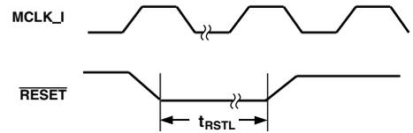
Figure 2. RESET Timing
