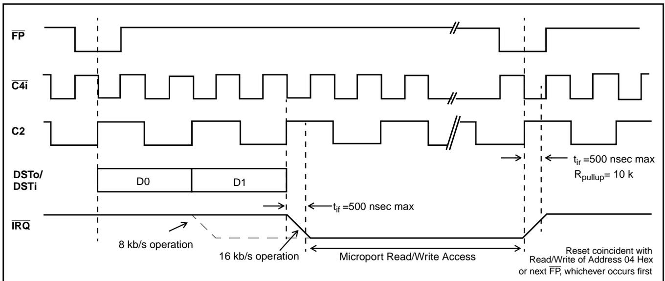
Figure 7b - IRQ Timing Diagram
