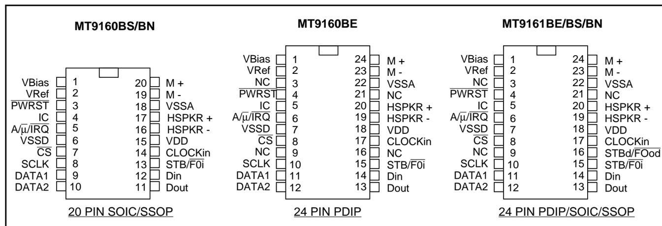
Figure 2 - Pin Connections
