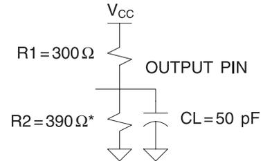
Note: Similar competitors' devices are specified with slightly different loads. These load differences may affect output signals' delay and slew rate. Atmel devices are tested with sufficient margins to meet compatible device specification conditions.
