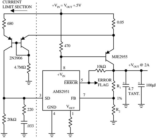
$$V_{OUT} = 1.23V(1+R_1/R_2)$$
