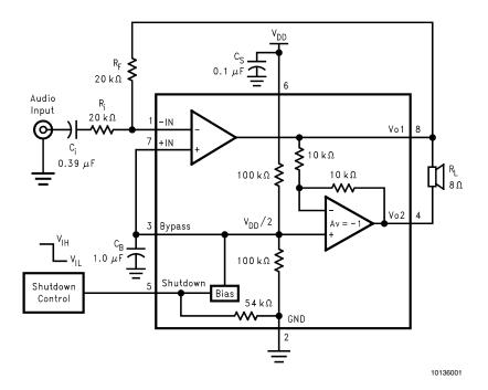
FIGURE 1. Typical Audio Amplifier Application Circuit
