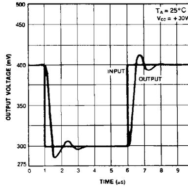
Fig. 9 LARGE SIGNAL FREQUENCY RESPONSE
