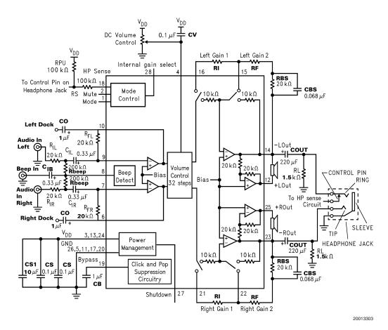
FIGURE 2. Typical Application Circuit ( LQ Package Pinout )
