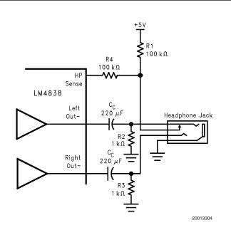
FIGURE 3. Headphone Sensing Circuit
