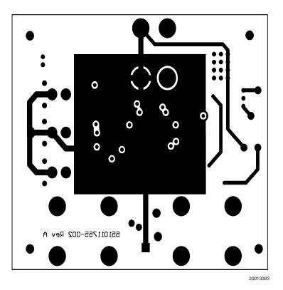
FIGURE 14. LM4838 micro SMD Bottom Layer
