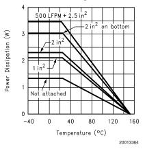
Note 18: These curves show the thermal dissipation ability of the LM4838MTE at different ambient temperatures given these conditions: 500LFPM + 2in<sup>2</sup>: The part is soldered to a 2in<sup>2</sup>, 1 oz. copper plane with 500 linear feet per minute of forced-air flow across it. 2in<sup>2</sup>on bottom: The part is soldered to a 2in<sup>2</sup>, 1 oz. copper plane that is on the bottom side of the PC board through 21 8 mil vias.
