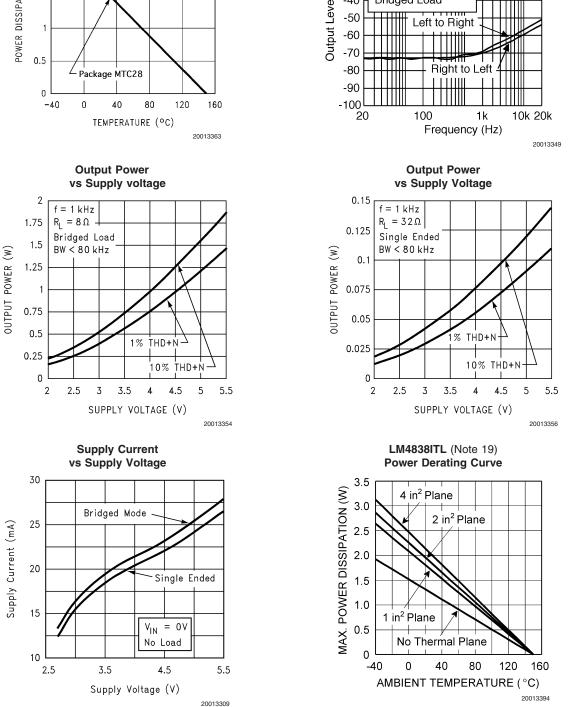
Note 19: These curves show the thermal dissipation of the LM4838ITL at different ambient temperatures with a thermal plane of size shown on an outside PCB layer using 1oz. copper.
