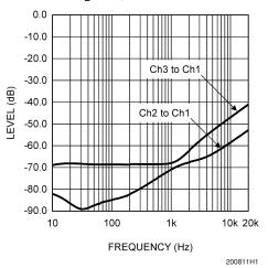
Crosstalk vs Frequency  $\pm 19V$ ,  $P_{OUT} = 10W$ , Channel 3  $R_L = 4\Omega$ , 80kHz BW
