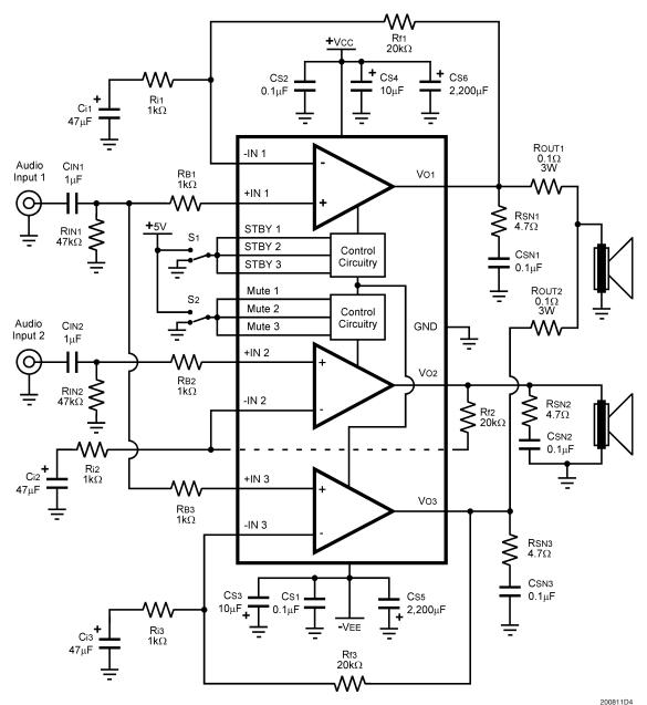
FIGURE 3. Parallel Amplifier Application Circuit
