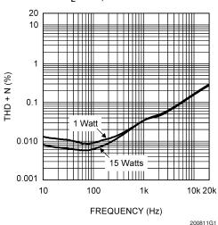
THD+N vs Frequency  $\pm 25$ V,  $P_{OUT}$  = 1W & 15W/Channel  $R_L$  =  $8\Omega$ , 80kHz BW
