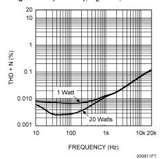
THD+N vs Frequency  $\pm$ 22V, P<sub>OUT</sub> = 1W & 40W, All Chs in Parallel Mode (Note 18), R<sub>L</sub> =  $2\Omega$ , 80kHz BW
