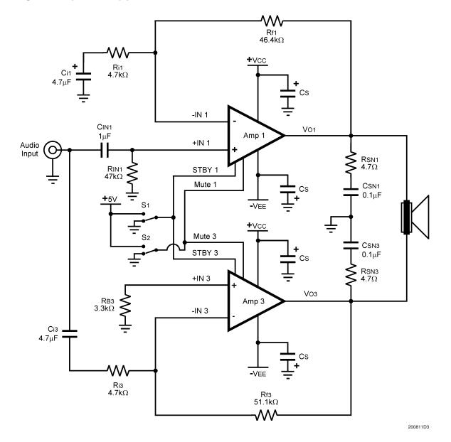
FIGURE 2. Bridged Amplifier Application Circuit
