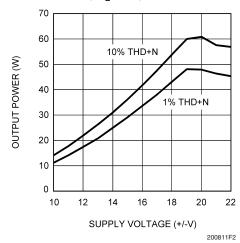
Output Power vs Supply Voltage All Chs in Parallel Mode (Note 18) f = 1kHz,  $R_L = 2\Omega$ , 80kHz BW
