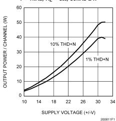
THD+N vs Output Power/Channel  $\pm 25V$ , R<sub>L</sub> =  $8\Omega$ , 80kHz BW
