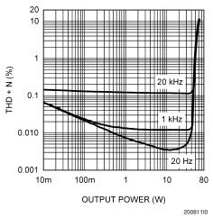
THD+N vs Output Power  $\pm 22V$ , All Chs in Parallel Mode (Note 18)  $R_1 = 2\Omega$ , 80kHz BW
