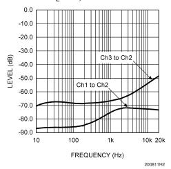
Two Channels On Crosstalk vs Frequency  $\pm 19$ V,  $P_{OUT} = 10$ W,  $R_L = 4\Omega$ , 80kHz BW
