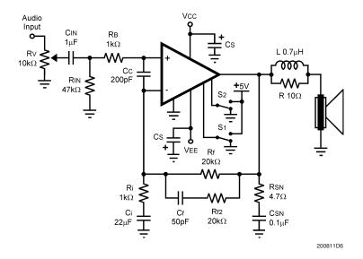
FIGURE 5. Special Audio Amplifier Application Circuit
