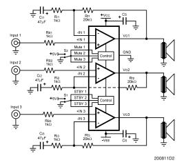
FIGURE 1. Typical Audio Amplifier Application Circuit
