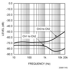
Crosstalk vs Frequency  $\pm 25$ V,  $P_{OUT} = 10$ W, Channel 3  $R_L = 8\Omega$ , 80kHz BW
