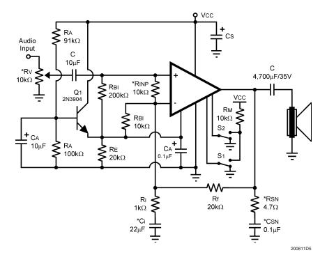
FIGURE 4. Single Supply Amplifier Application Circuit
