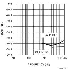
Two Channels On Crosstalk vs Frequency  $\pm 25$ V,  $P_{OUT} = 10$ W,  $R_1 = 8\Omega$ , 80kHz BW
