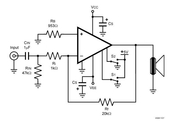
FIGURE 7. Inverting Amplifier Application Circuit
