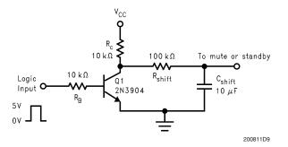
FIGURE 6. Level Shift Circuit
