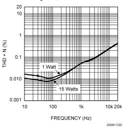
THD+N vs Frequency  $\pm$ 22V, P<sub>OUT</sub> = 1W & 15W/Channel R<sub>I</sub> =  $6\Omega$ , 80kHz BW
