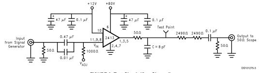
FIGURE 2. Test Circuit (One Channel)
